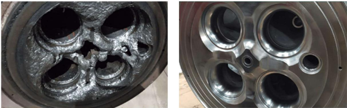
*A severely damaged cylinder head before and after refurbishment*
